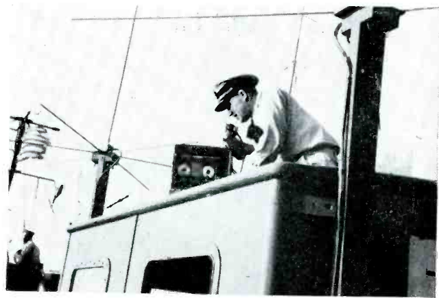
Lt. (jg) Dunbar aboard Navy cutter. Note the Abbott TR-4 and the end-fed antenna with counterpoise.
